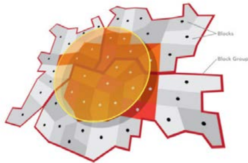
Figure 1: Illustration of the GeoEnrichment Tool - data apportionment for a 1-km ring around a location. Source: Esri
